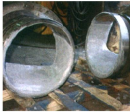
Repair/Line Chutes in Crushers with Wear Guard High Load
